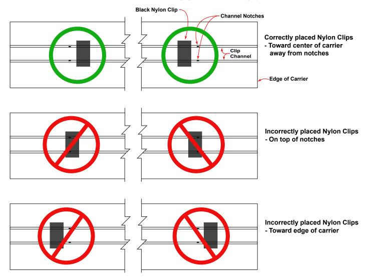
Once both black nylon carrier clip brackets have been installed properly on the back of the carrier, run an attaching strap through the slot of each nylon carrier bracket.
